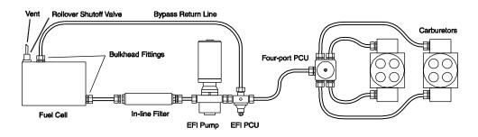
Note: To convert the ProStar SQ EFI Series pumps for carbureted application two regulators are necessary. A return style at the pump (MP-9950-C) which controls the pump pressure and a deadhead style at the carburetor to control pressure to the needle and seats.
