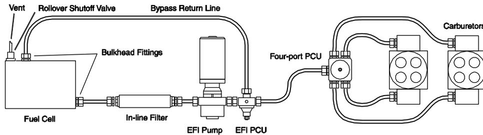
Note: To convert the ProStar EFI Series pumps for carbureted application two regulators are necessary. A return style at the pump (MP-9950-C) which controls the pump pressure and a deadhead style at the carburetor to control pressure to the needle and seats.
